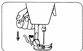
When you fail to catch the foot, push the lever in the arrow direction slightly.
